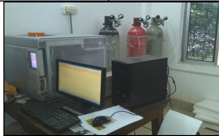
Fig. 15 Biogas check analyzer
