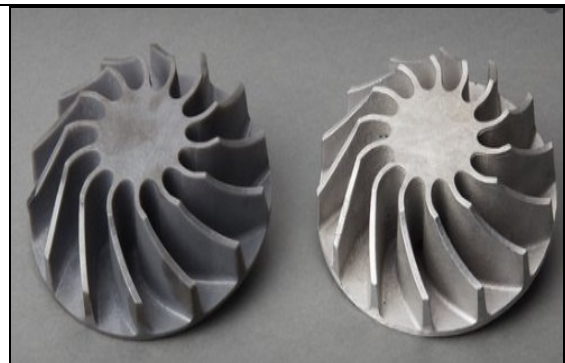
Figure 6 Comparison of Casting and ABS pattern
