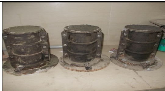
Fig 5: The cylinders after casting after mixing with different % of substitute of FeCr granules
