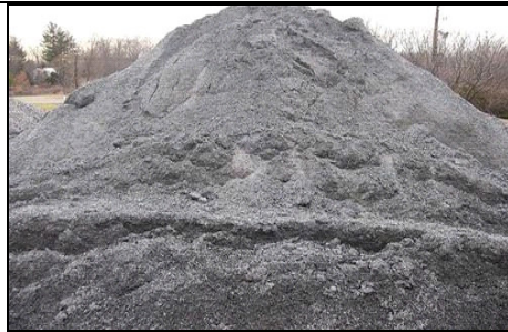
Fig 1: The fine particles of FeCr slag at Balasore Ferro alloys Ltd, Somoa
